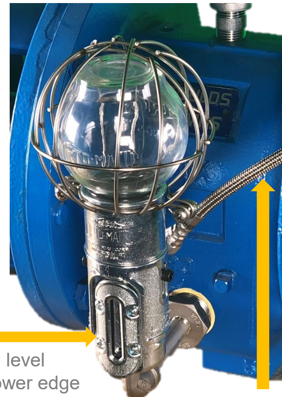
Pressure Balancing Line
